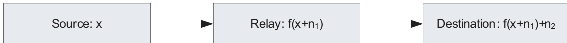
Figure 32: Finding the optimum relaying function f(r) .
